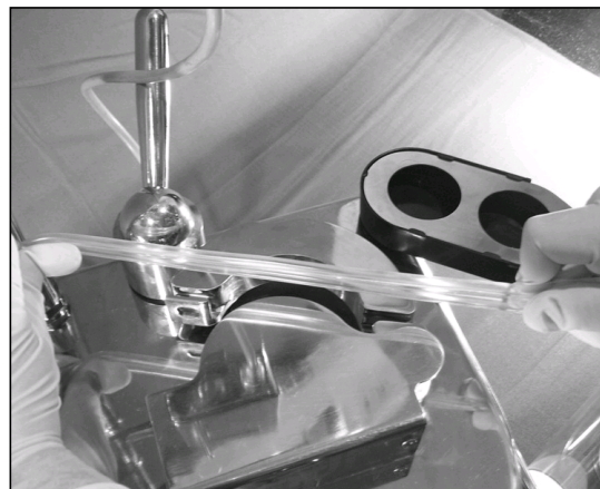
Pic. 4: Placement of PVC tubing in the Steripump head
